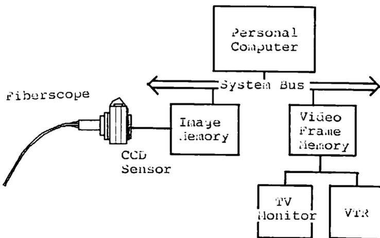
Figure 1 Block diagram of image recording system.
