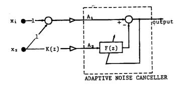
Fig. 4 Single-channel adaptive noise canceller without noise in the inputs. The sources x<sub>1</sub> and x<sub>2</sub> correspond to 'T-complex' and 'nonspecific response', respectively, in Walpaw & Penry's model on auditory evoked responses of temporal cortex (A<sub>1</sub>) and vertex (A<sub>2</sub>).
