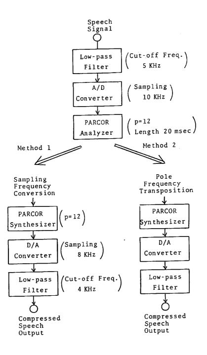
Fig. 1. Schematic diagram of the frequency compression. The parameter values used in the preliminary listening test are shown in parentheses.
